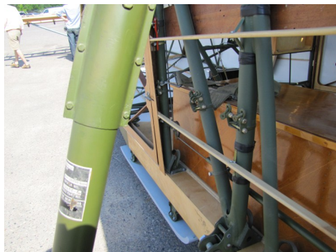
The craftsmanship is superb! It was a great idea to leave a side off so all the parts are visible without climbing into the glider. (Surprising that Viqueens fans would think of something like that!) Basic instruments. Tie downs behind the seats were used to secure Jeeps, Pack Howitzers and mortars and small bulldozers. The quality stamp on the tail part at left shows it came from Marshfield. (Laney Pics)
